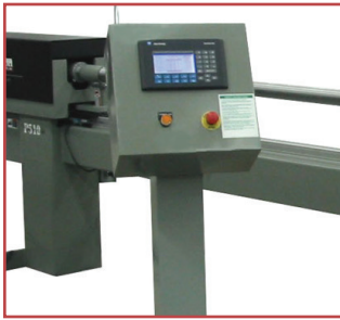
Free-Standing Allen-Bradley PanelView touch-screen controls
