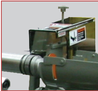
Double guarded fixed knife for operator safety
